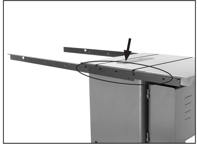
Figure 13. Rear rail installed.
